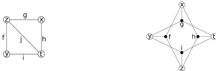
Figure 2.1: The rule replace x, y, z, t by P(x, y, z, t) if f(z, y) \wedge g(x, z) \wedge h(x, t) \wedge i(y, t) \wedge j(z, t) has an arity of 4 and a rank of 2 and can be represented as a graph (left). The rule replace x, y, z, t by P(x, y, z, t) if f(x, y, z) \wedge g(x, y, t) \wedge h(x, z, t) \wedge i(y, z, t) has an arity of 4 and a rank of 3 and needs a hypergraph to be represented (right).
