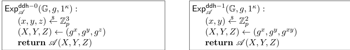
Figure 2.4: Experiments \text{Exp}_{\mathcal{A}}^{\text{ddh}-0}(\mathbb{G}, g, 1^\kappa) and \text{Exp}_{\mathcal{A}}^{\text{ddh}-1}(\mathbb{G}, g, 1^\kappa) for the decisional Diffie-Hellman problem over a group \mathbb{G} with generator g
