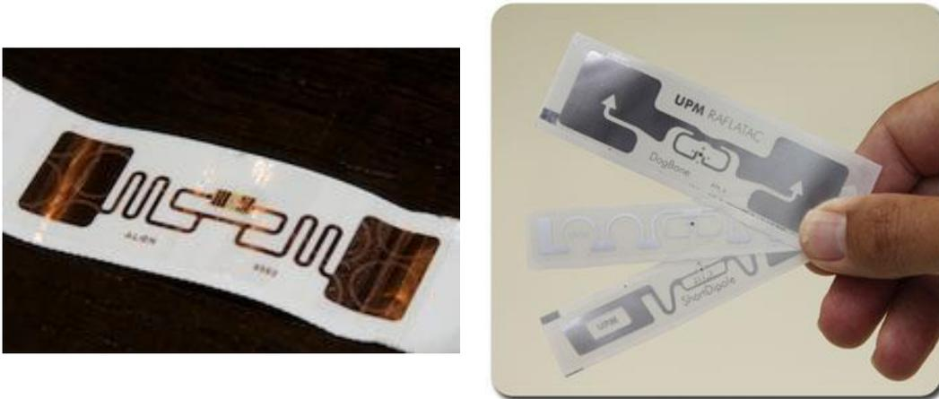
*Figure I.4: Disposable RFID tags used for race timing.*
