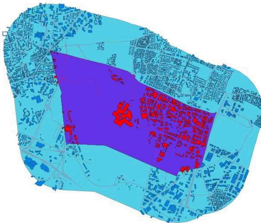
Figure 4: Representation of the building point of view. The geographical area of interest is in purple. This is where the buildings' façades will be evaluated. The blue zone is the width of the outside buffer of d_{max} (1000m).
