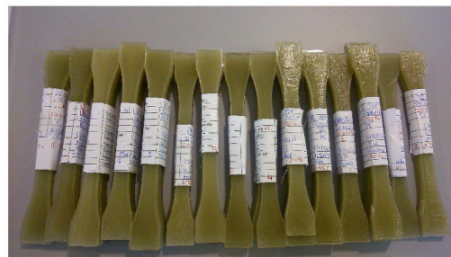
(b) 3DP samples with a degradation of four 3D printing processes
