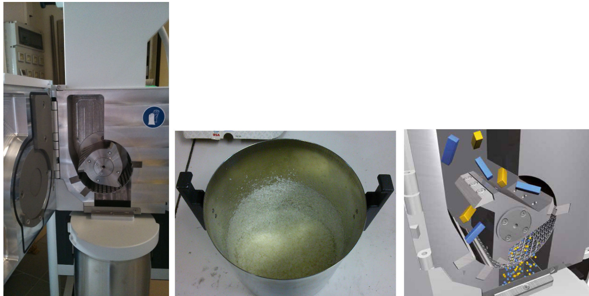
Figure 4.28: Machine used for the recycling process
