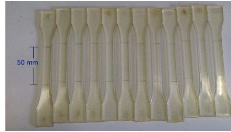
(b) Marks in the samples in order to attach the extensometer
