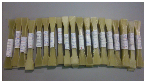
(a) Filaments made from first recycling cycles (b) 3DP samples with a degradation of two 3D printing processes
