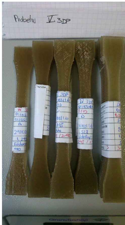
(b) 3DP samples with a degradation of five 3D printing processes
