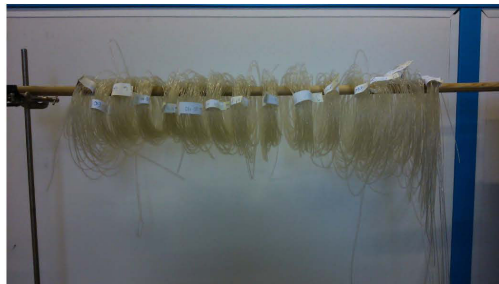
(a) Filaments made from the second recycling cycle
