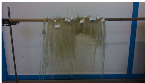
(a) Filaments made from the third recycling cycle
