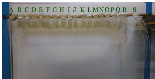
(a) Filaments made from first recycling cycles (b) 3DP samples with a degradation of two 3D printing processes
