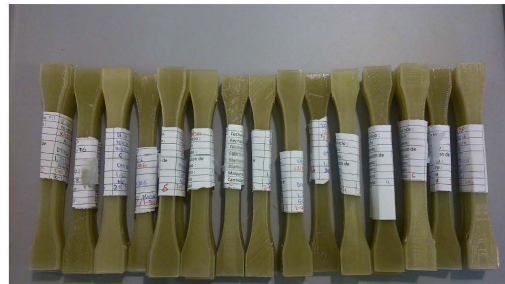
(b) 3DP samples with a degradation of three 3D printing processes
