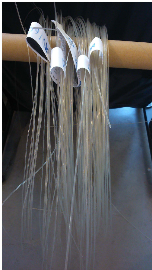
(a) Filaments made from the four recycling cycle
