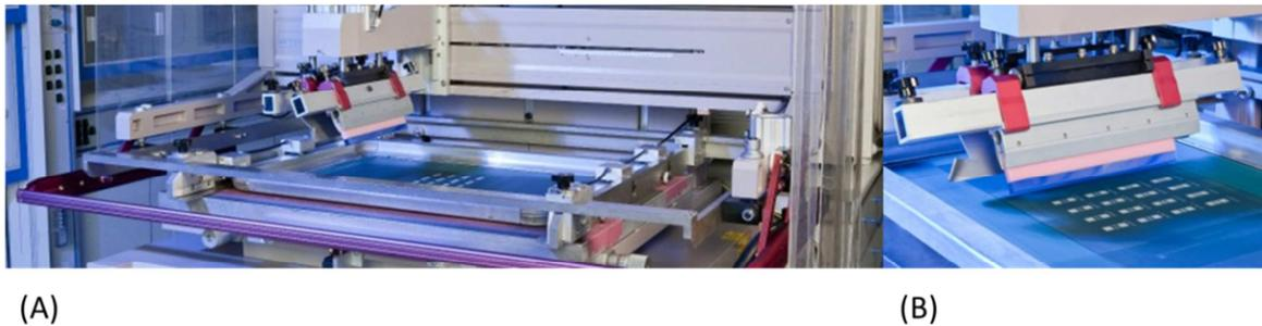
Figure 1.4 (a). (b). Screen printer using Clevios™ ink [Reproduced with permission from Heraeus]
