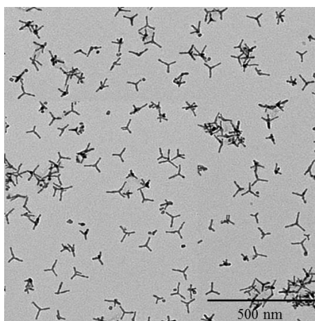
Figure 2.23 : TEM image of PdCu tripods.
