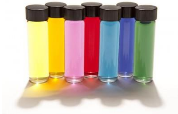
Figure 2.1 : The intense color of gold nanoparticles arises from surface plasmon resonance modes, resulting in photon absorption at various wavelengths.
