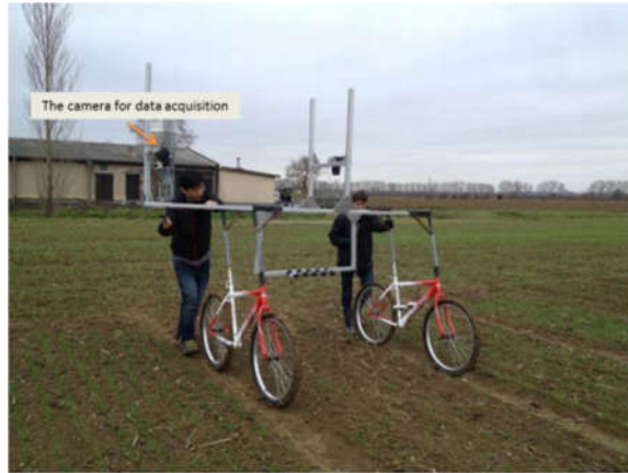
Fig. 1 The image acquisition in the field with the Phenotypette
