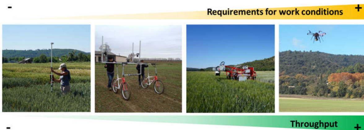
Fig. 3 Different types of phenotyping systems. From left to right, it corresponds to portable instrument, semi-automatic platform (Phenotypette), automatic field robot (Phenomobile) and unmanned aerial vehicle (UAV).
