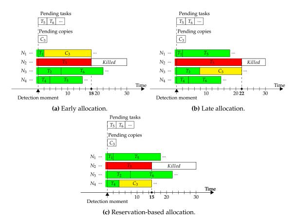
**Figure 6.3** – An example with different speculative execution mechanisms.
