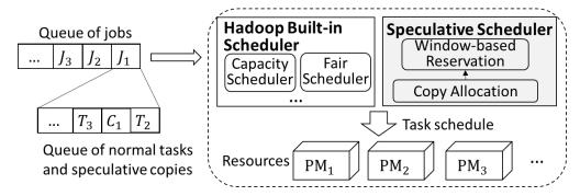
Figure 6.4 – Design overview of the reservation-based speculative execution mechansim.
