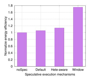
**Figure 6.10** – Energy efficiency with different speculative execution mechanisms.
