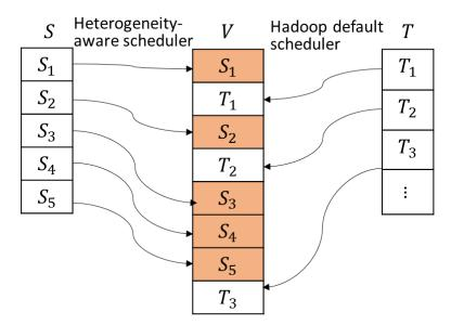
**Figure 6.5** – An example of window-based resource reservation. In the current window, *S* is the set of detected stragglers ordered by criticalness, *V* is the set of available slots and *T* is the set of regular tasks to schedule.
