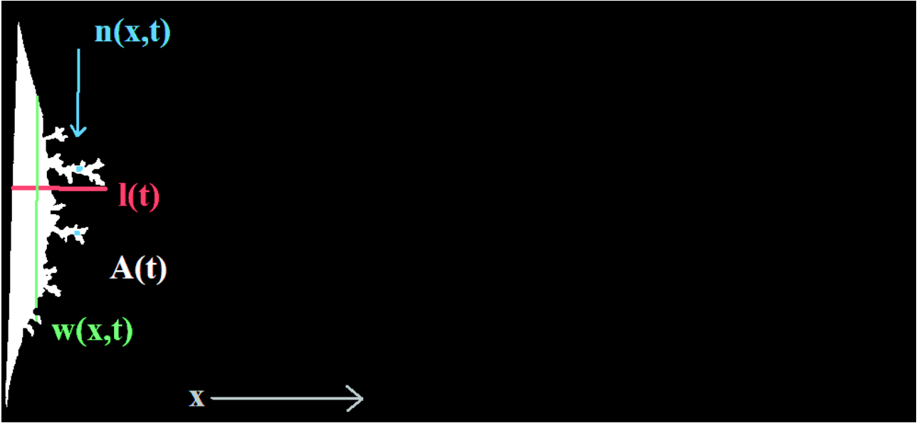
Figure 6: Indications of the measurable quantities of the pattern: the total width w , area A , length of the most advanced finger l and the number of fingers n . The "1" pixels are white and the "0" pixels are black. The x -direction is from the closed short-side toward the semi-permeable short side, and the time t is the experimental time of the frame.
