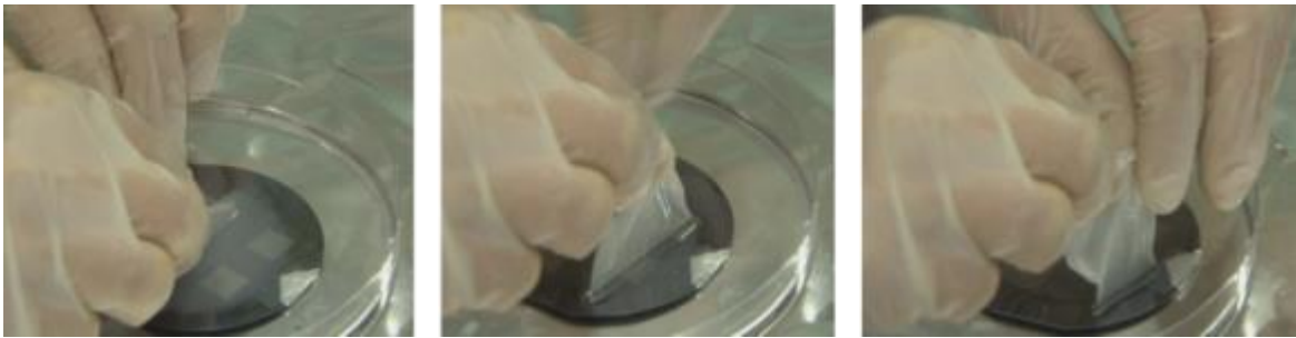
Figure S1: Peeling operation to remove the membrane from the micropatterned collector
