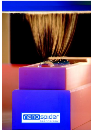
Figure 6: Needleless electrospinning system presented by Elmarco Co.
