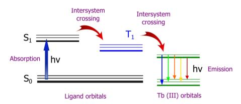
Figure 18. Principle of the Tb (III) luminescence.
