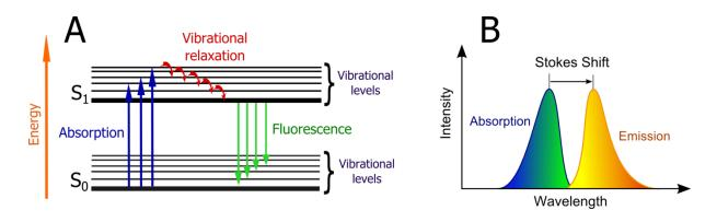
**Figure 16.** (A) A simplified representation of the Jablonski diagram of molecular energy levels. (B) A schematic representation of absorption and emission spectra.
