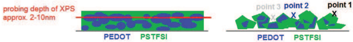
Fig. 2.18: Schematic illustration of the difference for XPS measurements on film and on powder
