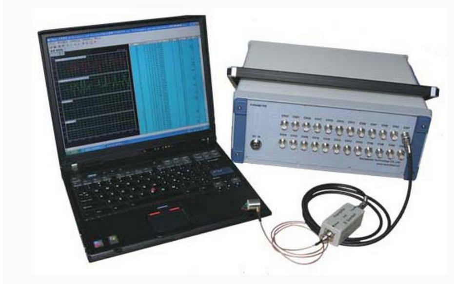
Fig. 6.2 Acoustic emission monitoring equipment.
