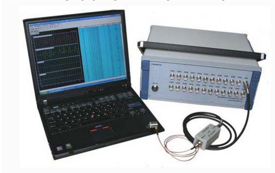
Fig. 6.2 Acoustic emission monitoring equipment.
