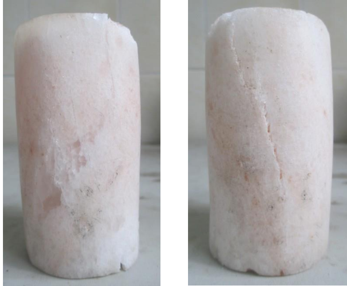
Fig.2.11 Specimen failed in the uniaxial test
