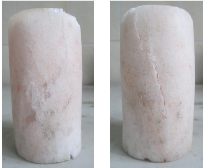
Fig.2.11 Specimen failed in the uniaxial test
