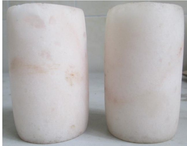
Fig.2.18 Deformed salt rock specimen before D point from trial tests
