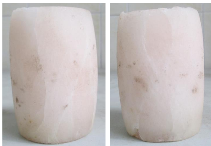
Fig.2.19 Fractured salt rock specimen after D point from trial tests
