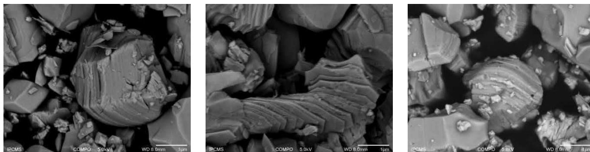
Figure III.16. SEM images of alkyne-HST (left), hexyl-click-HST (middle) and benzyl-click-HST (right).
