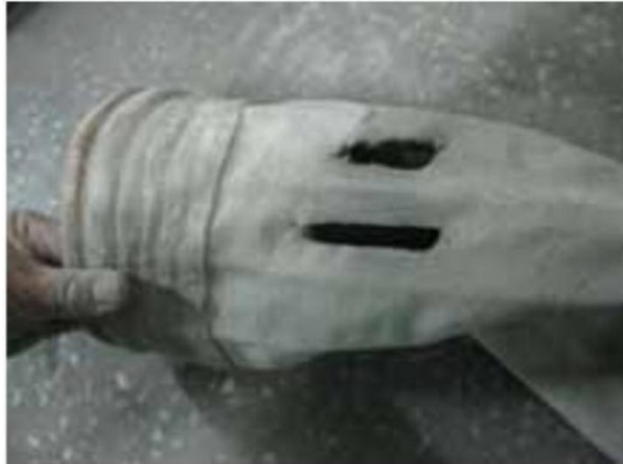
Figure 19: Damaged bag filter (Zhou et al. 2012)
