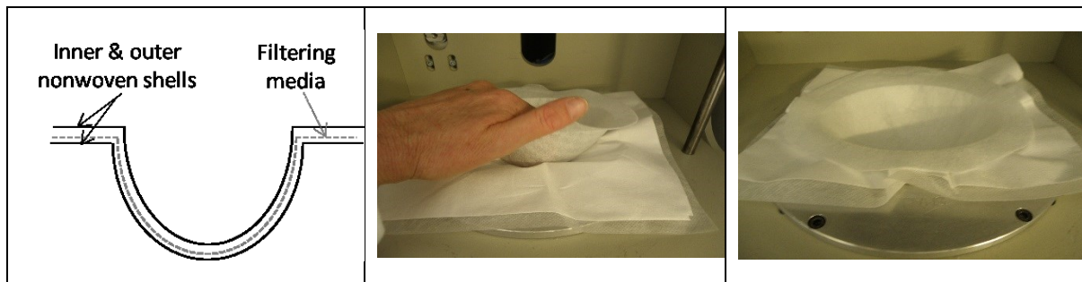
Figure 40: Molded filters developed from PA-6 nanofibers sandwiched between nonwoven layers
