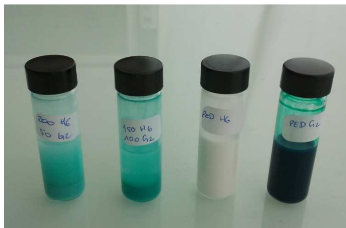
Figure 17: Acid base interactions between hybrid particles. From the right to the left side: acid PED G2 (P.G./Poly(AA-co-LA 32 )) , basic PED H6 (TiO 2 -DTS/Poly(4-VP-co-LA 26 )), a mixture of PED H6 (150 mg) and PED G2 (100 mg) and an other mixture of PED H6 (200 mg) and PED G2 (50 mg)
