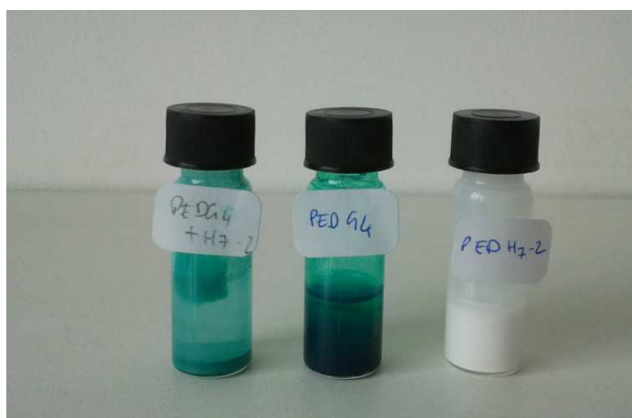
Figure 18 : Acid base interactions between hybrid particles. From the right to the left side: acid PED G4 (P.G./Poly(AA-co-LA 98 )) , basic PED H7-2 (TiO 2 -OTS/Poly(4-VP-co-LA 69 )), a mixture of PED H7-2 (150 mg) and PED G4 (100 mg)
