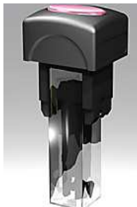
Figure 1: The dip cell used to measure solution in non polar media [3]
