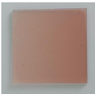
Figure 10 : Picture of the NP 80:20 PC 71 BM:PCDTBT sprayed onto ZnO substrate
