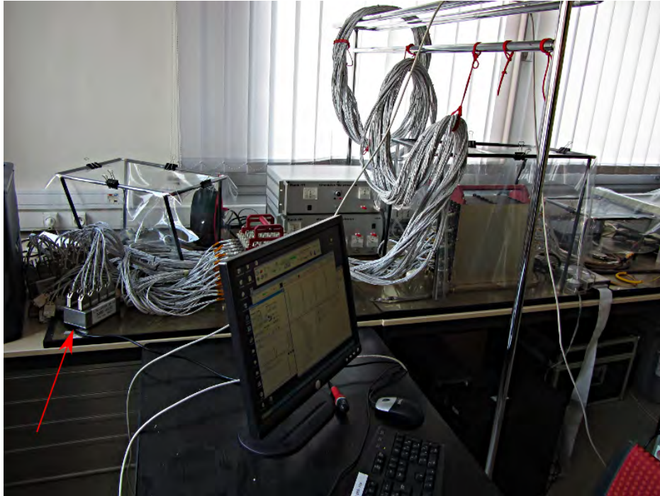
Figure 4.15: Photo of the HFI electronics flight spare taken at IAS in February 2012. The red arrow points to the box housing the load resistance used instead of bolometer, and the software used for data acquisition is visible on the foreground LED screen.
