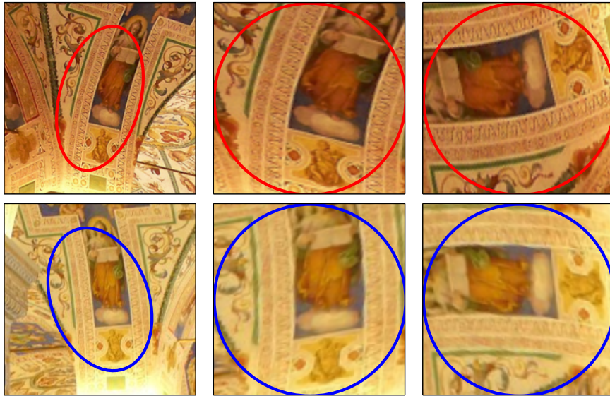
Figure 3.6: Example of matching points in two different images. Salient points are extracted (left), affine rectified (middle), and normalized in rotation (right). Note that the level of invariance which remains to be covered by the patch descriptor is relatively low, as most of the work has been accomplished by the detector.
