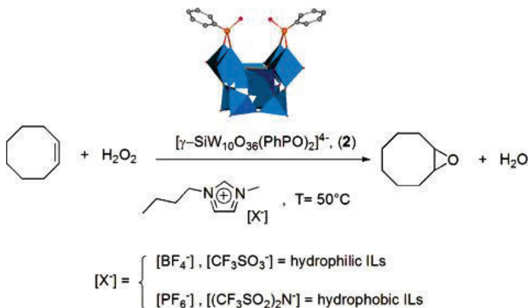
Figure 2. 11- Catalytic epoxidation of cis -cyclooctene by the hybrid POM with \text{H}_2\text{O}_2 in ILs, proposed by Berardi et al.
