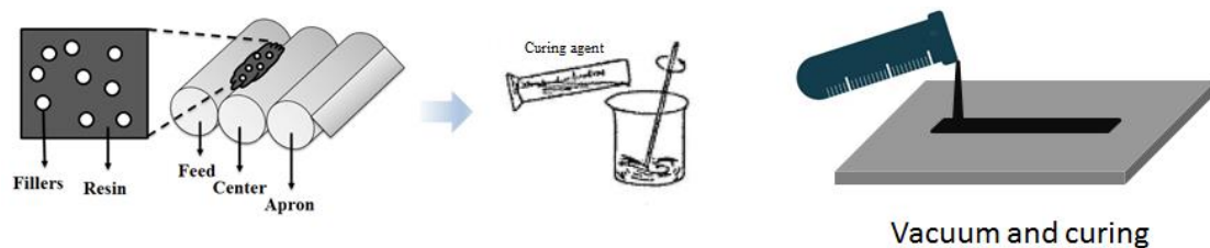
Figure 4.1 Three-roll milling method process to prepare the epoxy composites with graphene-based nanofillers.
