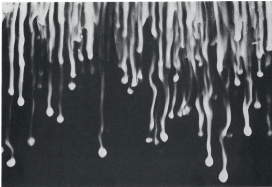
FIGURE 1.1: Visualization of salt fingers in a laboratory experiment. A salty solution is poured at the top of a liquid with stable temperature gradient. The downward-moving fingers are made visible by adding fluorescein to the salt and lighting through a slit from below. Taken from Huppert and Turner (1981a) .
