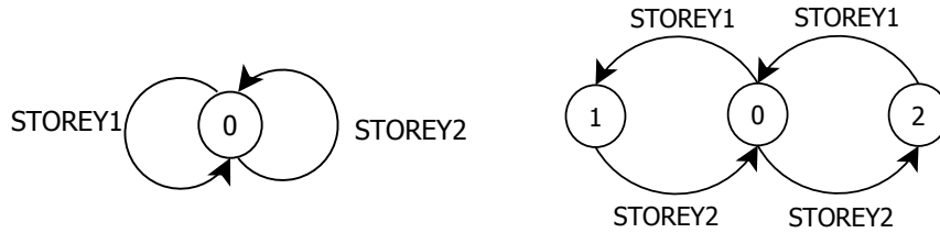
Figure 6.2: LTSs describing activation policies of Storey1 and Storey2
