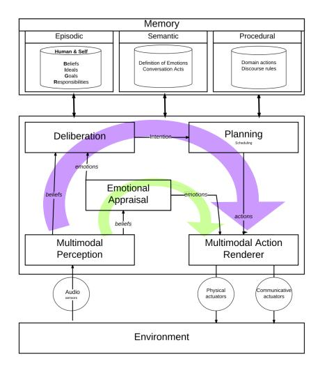
FIGURE 5.1: The CAIO architecture.
