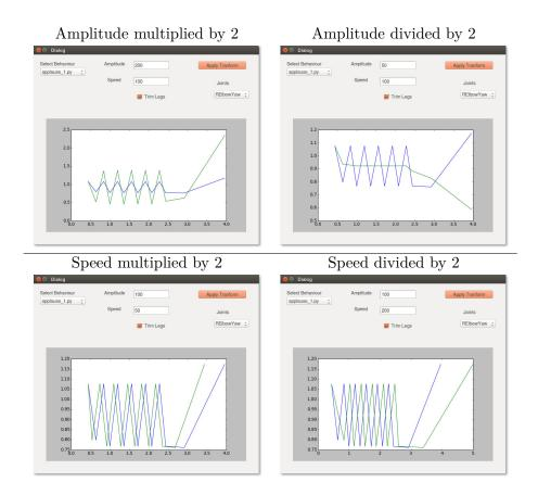
**FIGURE 4.11:** Examples of motion transformations of the Elbow-raw joint when clapping, where the blue line is the same original motion and the green lines are the computed new motions
