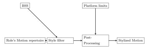
FIGURE 4.5: Pipeline of Stylistic treatment of data
