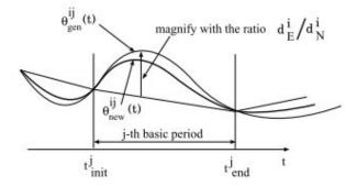
FIGURE 4.9: Amplitude transformation of joint angles from [Amaya et al., 1996]
