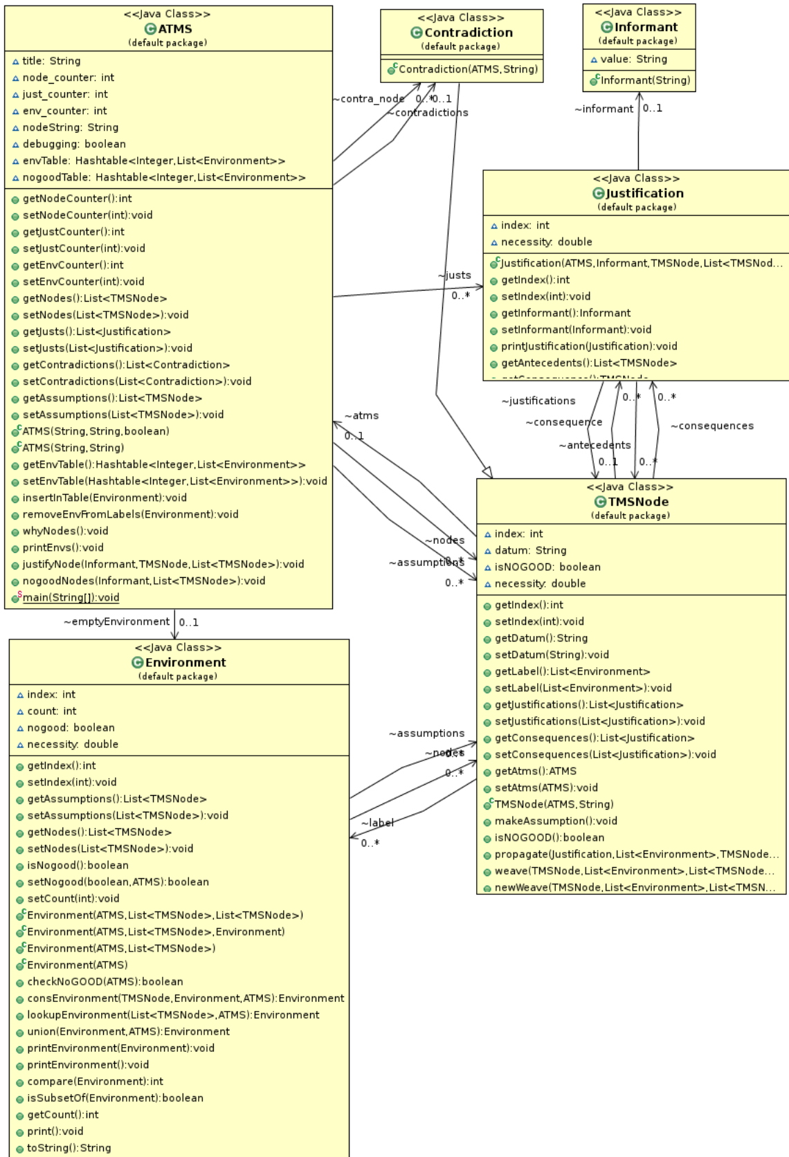
Figure 5.4: ATMS class diagram.
