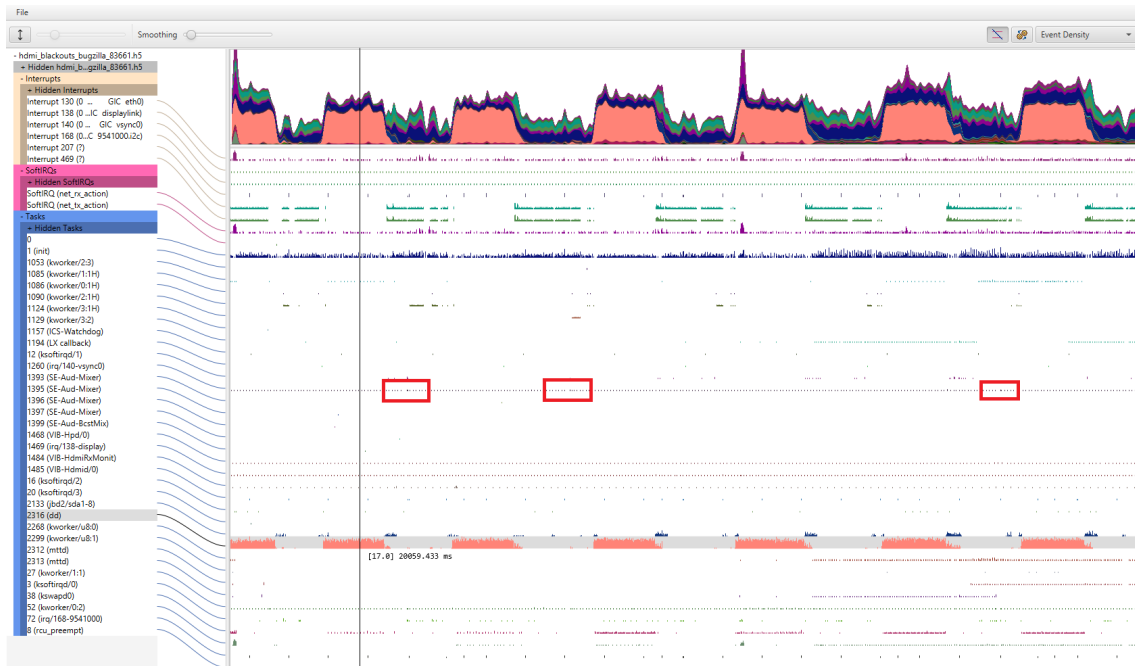
Figure 7.8: TraceViz showing an execution when video blanks appeared. The system is artificially loaded with heavy some I/O using the dd Unix command, represented in orange. The task jbd2-sda1-8 is scheduled directly after the dd task, causing delays on the treatment of the VSync IRQ callback, in the red rectangles.
