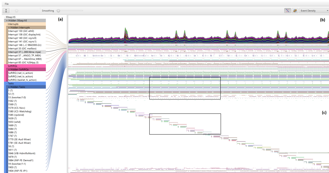
Figure 7.4: Overview of TraceViz. TraceViz interface consists of three main areas: the tree view (a), the outline view (b), the timeline view (c) and the links that connect the actors and their corresponding graphs (d).
