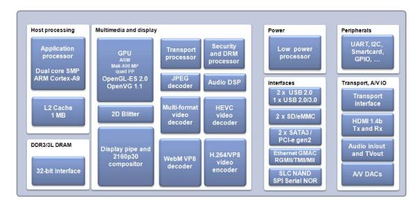
Figure 2.2: Block diagram of the STMicroelectronics Monaco MPSoC for set-top boxes. Each block represents a dedicated chip for a specialized task.
