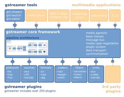
Figure 2.4: GStreamer architecture overview [GStreamer, 2016]
