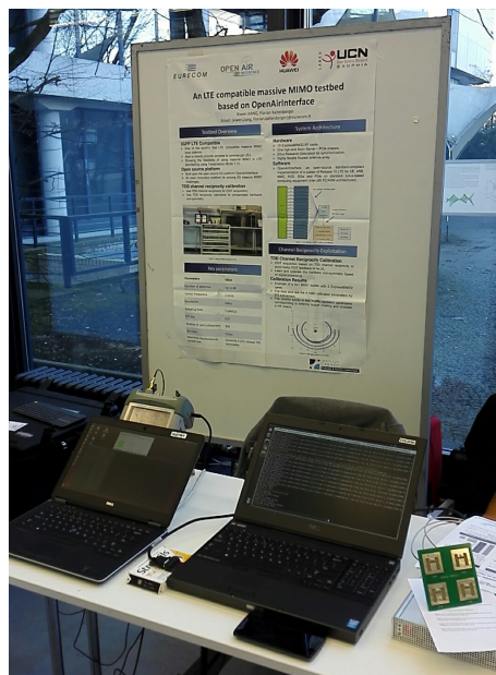
Figure 10.22: A scaled-down version of massive MIMO prototype with 4 antennas demonstrated in WSA Berlin showing the interoperability with commercial UE. TDD reciprocity calibration is used for CSIT acquisition. The system then performs MRT beamforming to the UE for Internet service.
