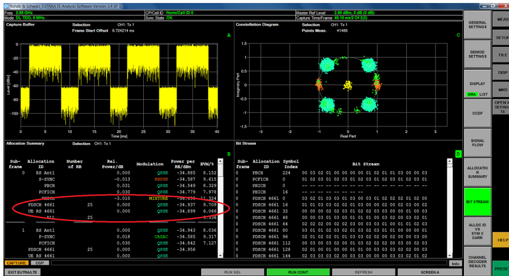
Figure 10.17: Validation of the TM7 implementation using Rohde & Schwarz FSQ Signal Analyzer
