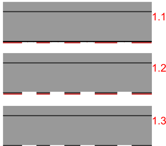
FIGURE 5.10: Process steps for patterning the hard mask in the backside.
