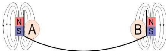
FIGURE 1.10: Holding principle via permanent magnet.
