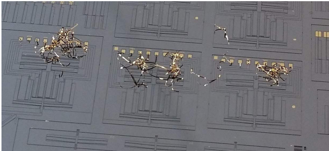
FIGURE 5.17: The gold patterns started to peel off from the wafer after inserting it in the HF solution.
