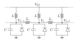
**Figure 3.5:** Electrical analogue of the excitable Burridge-Knopoff model as a nonlinear transmission line.
