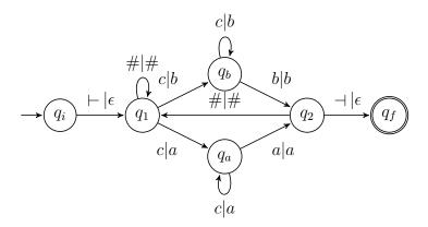
Figure 2.10: A one-way non-deterministic transducer  $\mathcal{H}'$  computing h'.
