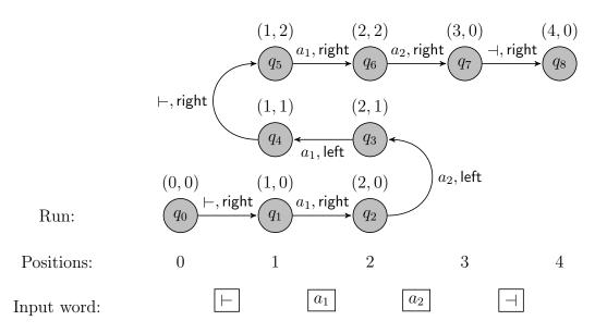
Figure 2.1: Graphical presentation of a run of an automaton.
