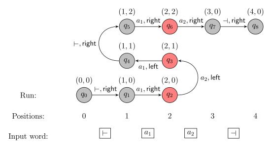
**Figure 2.2:** The crossing sequence at position 2 is  $(q_2, q_3, q_6)$
