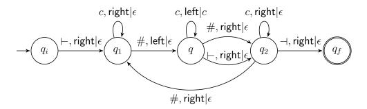
Figure 2.7: A transducer  $\mathcal{G}'$  representing the function g'.
