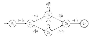
Figure 2.9: A one-way non deterministic transducer  $\mathcal{H}$  computing h.
