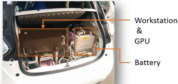
Figure 4.2 – Computing facilities on the ZOE
