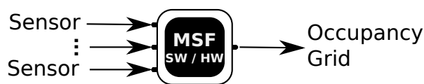
Figure 1.5 – The Multi-sensor Fusion (MSF) module composed of sensors and a software (SW) and hardware (HW) integration of MSF
