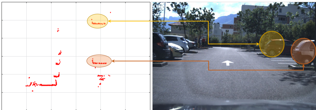
Figure 4.4 – Scan points of an ibeo LUX LIDAR mounted on the front bumper of the prototype car (image courtesy of INRIA Rhône-Alpes)
