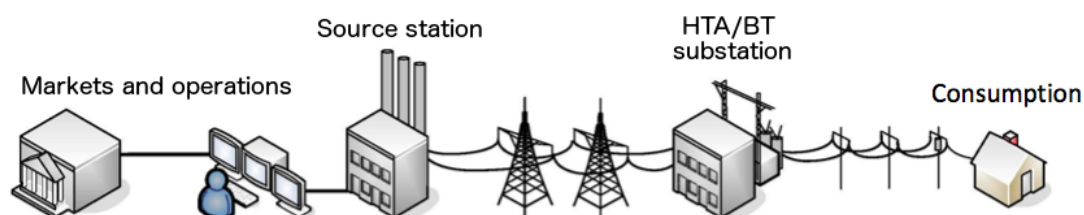
Figure 6.1 – Simplified view of a power grid
