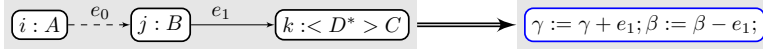
Figure 8.2: An example of LDRS where the first \beta after an \alpha on a path toward a C becomes a \gamma . The dashed line represent the program \alpha and the plain line the program \beta .
