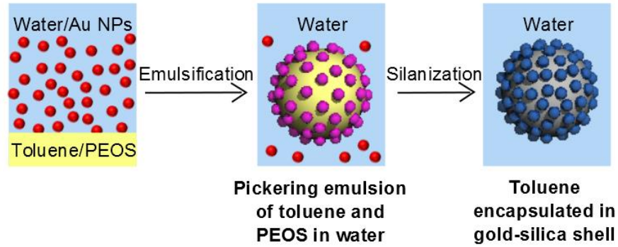
Figure 84: Schematic representation of the formation of gold-silica microcapsules.
