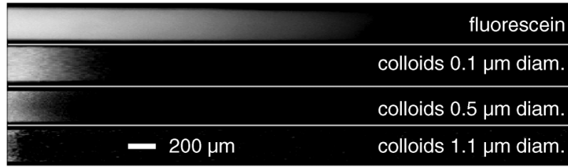
Figure 36: Evaporation-induced concentration of different sizes of solutes 69 .
