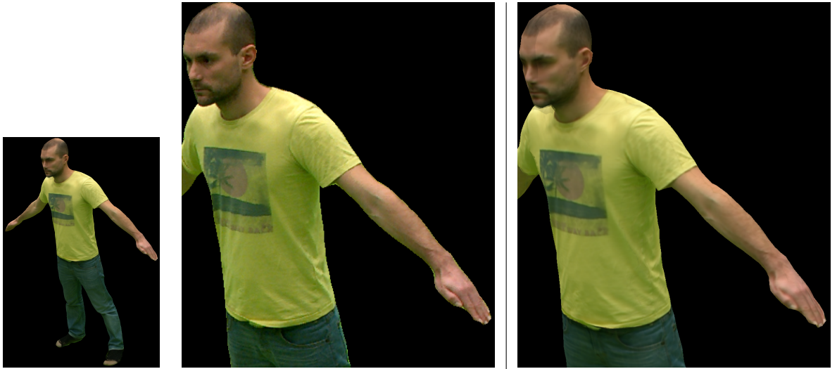
Figure 3.6 – From left to right: Computed image with the weighted arithmetic mean texture map through the observation model \hat{I}_i = \mathbf{P}_i \hat{\mathbf{T}}_{\text{mean}}^{\text{weighted}} . Close ups on the T-Shirt and face of input and computed image. Due to the weighting scheme appearance candidates from cameras who are not fronto-parallel to the object have a smaller weight in the computation of the appearance and thus previous artifacts on the T-shirt are eliminated.
