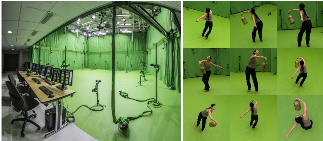
Figure 2.1 – Kinovis platform, at Inria Grenoble. Left: acquisition room. Right: simultaneous images from a subset of cameras.
