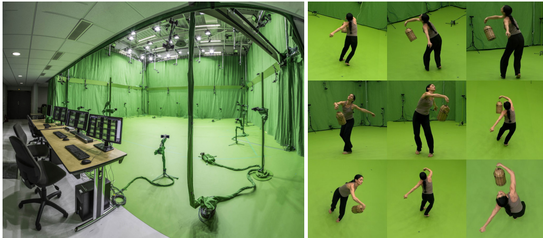
Figure 2.1 – Kinovis platform, at Inria Grenoble. Left: acquisition room. Right: simultaneous images from a subset of cameras.
