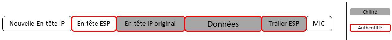
FIGURE 5.2 – IPsec en mode tunnel.
