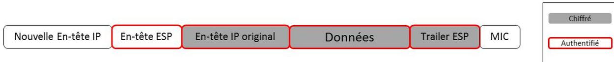
FIGURE 5.2 – IPsec en mode tunnel.
