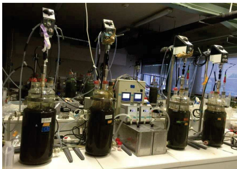
Figure 11: Four 6 litres CSTR reactors
