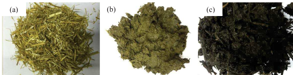
Figure 10: Substrate of reactors: (a) straw (R1), (b) cow dung (R2) and (c) cow manure (R3, R4)
