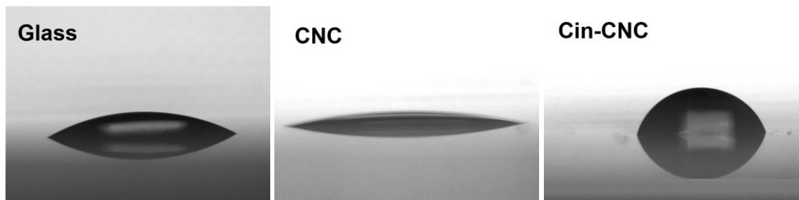
Figure 6.6. Images of the water droplets deposited on the glass support, before and after spin-coating with the CNC and Cin-CNC material.
