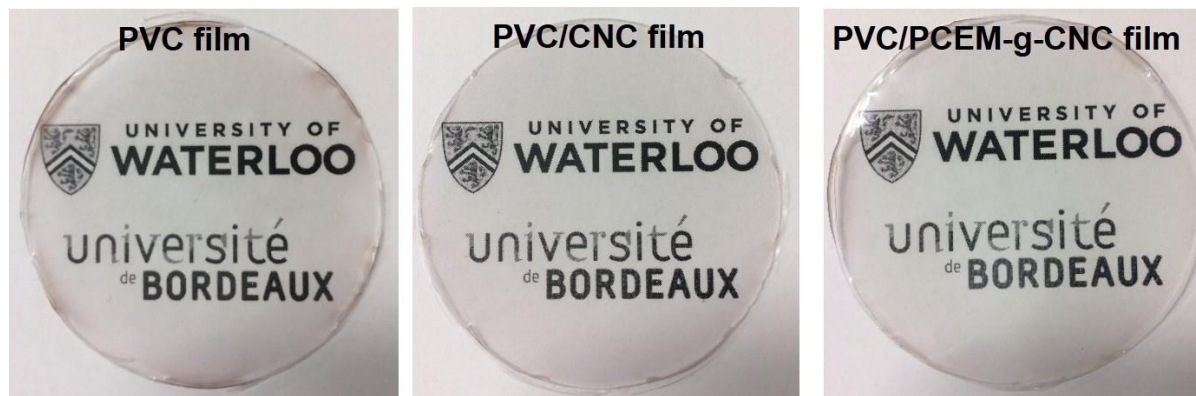
Figure 5.8. PVC, PVC/CNC (5 wt. %) and PVC/PCEM-g-CNC (5 wt. %) composite films obtained by solution casting of the corresponding DMF solutions/suspensions followed by heat annealing.
