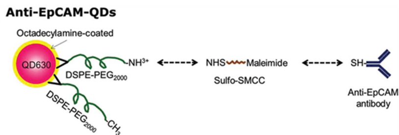
Figure 1-8. Construction of anti-EpCAM antibody-conjugated quantum dots (anti-EpCAM-QDs) as primary nanoparticles. DSPE-PEG 2000-methoxy and DSPE-PEG 2000-amine were grafted onto the surface of the QDs and the resulting QDs and antibodies were conjugated using a sulfo-SMCC linker. 39
