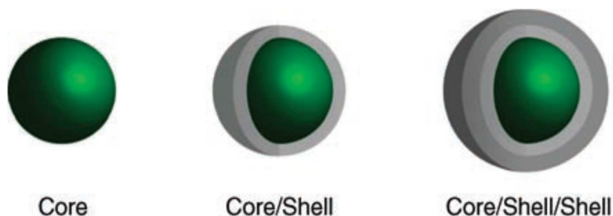
Figure 1-3. Illustration of core, core/shell and core/shell/shell QDs. 14
