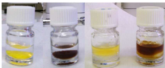
Figure 2-5. Mutual colour change of the chloroform phase (bottom) and aqueous phase (top) during phase transfer. Yellow sample: QD530 ; brown sample: QD705 .
