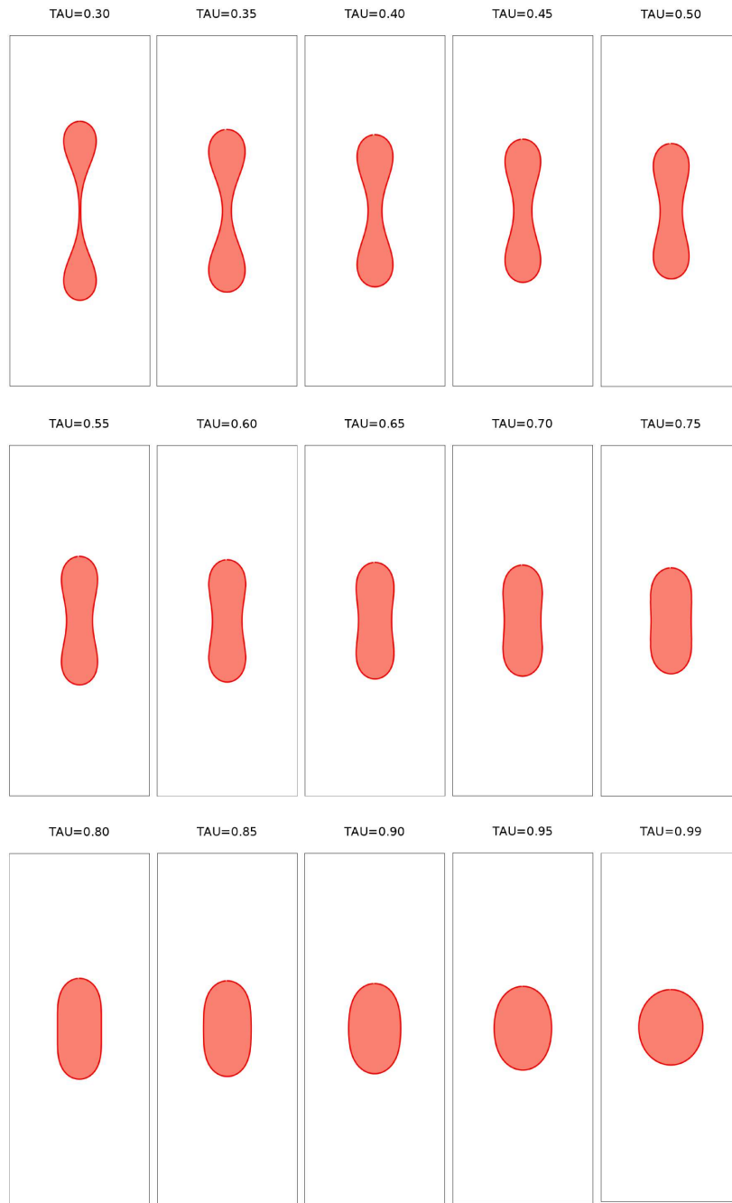
Figure 3.4: Shape transformation of a vesicle as a function of the reduced area in a static fluid computed using 3.42 .
